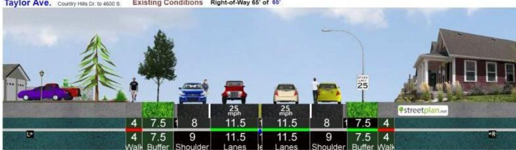
This rendering shows an example of how Taylor Ave. could be redesigned. The bottom rendering is the existing conditions on the street, and the top rendering is a potential reconfiguration of existing right-of-way space, including narrower driving lanes and new bike lanes to slow vehicle speeds, while still retaining on-street parking for residents.
