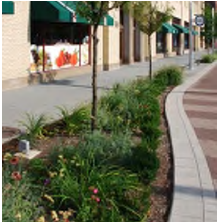
Sustainable stormwater streetscapes include rain channels, planted verges, and porous paving
